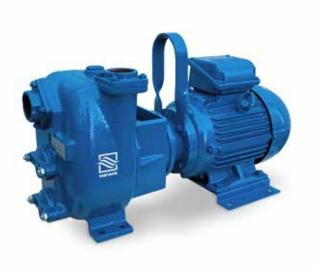
**Product Data** Suction port Threaded - 1 1/2" ISO 228 (BSP) Delivery port Threaded - 1 1/2" ISO 228 (BSP) Qmax 25 m<sup>3</sup>/h - 416 l/min (110 USgpm) Hmax 53 m (174 ft) Solids handling 11 mm (0.4 ") Motor power 7,5 kW - 10 HP Motor type **IEC** standard Winding for inverters **Cast iron frame** Motor brand WEG W22 Premium Weight 120 ka
